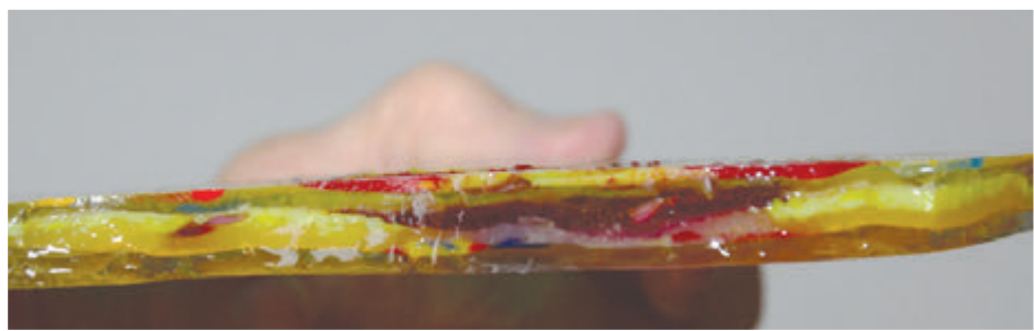
The final outcome of a piece is dependent to a large degree by its eventual thickness. Too few fused layers and it will break, to heavy and thick and the piece will become just a blob. Here can be seen several layers of fused glass at a desired ¼ of an inch thickness.
